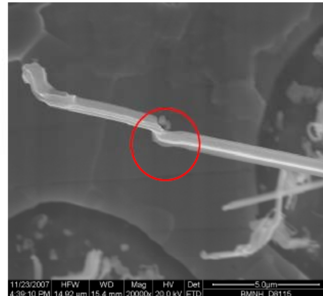
Storage at room temperature in air for 820hr, on the surface of CeSn 3 phase
